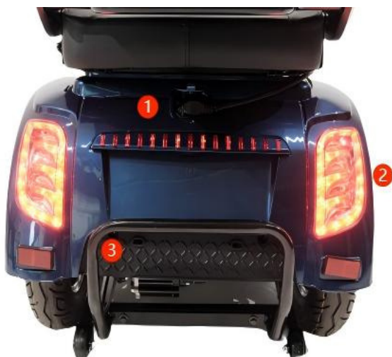
1: Charging port 2: Rear tail light 3: Rear Crash Bar
